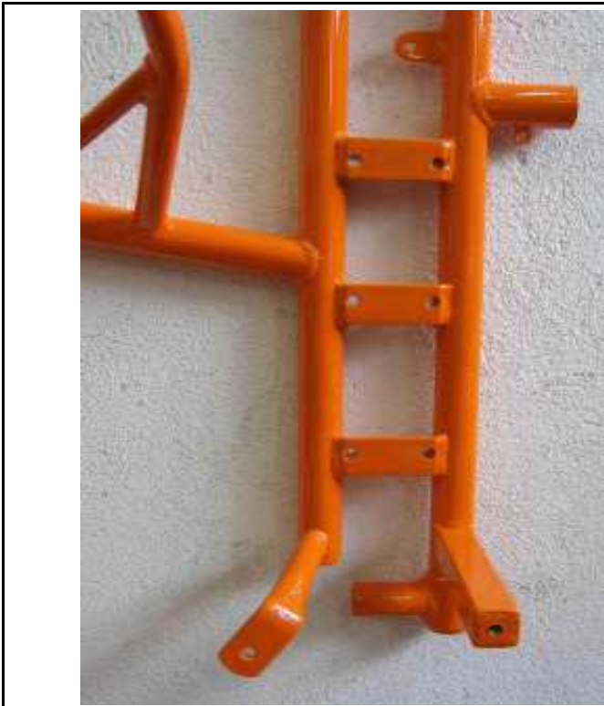
Foto from above of the frame with the section of the engine mount
